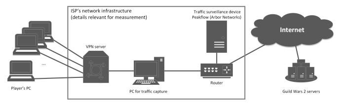
Fig. 1. Measurement setup
